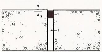
Example of sealed expansion joints in granolithic screeded areas is shown below.
